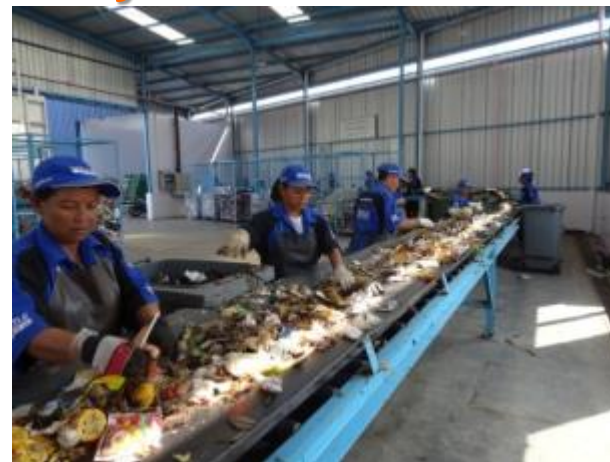
Intermediate waste separation facility (Surabaya)
